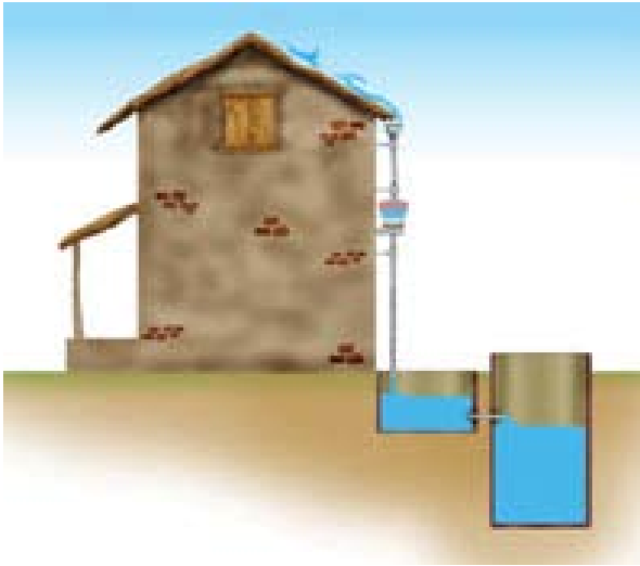
Example of Rain Water Collection System
